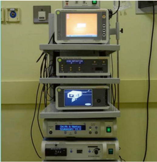
Fig. 71.2 Arthroscopy column. It includes screen, light source, video recording device, shaver water pump, and electrothermal system
